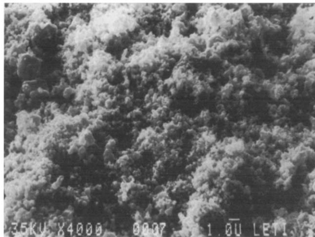
Fig. 3 Japanese 700Å powder sintered at 160°C: Sample J7(160). Scale (1 \mu\text{m} ) given by the white line
